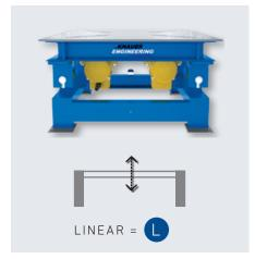
Two unbalance motors (external vibrators) which operate synchronous and in opposite direction create a linear movement of the table top. The result is a vertical directed harmonic oscillation.
